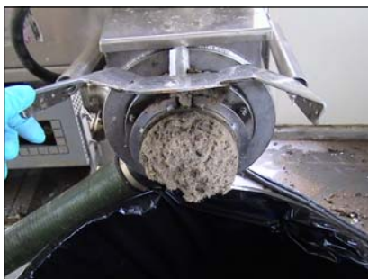
The dewatered screenings will pass the Paint Filter Test. They are generally suitable for land filling; they have also been used as fuel for cogeneration.
