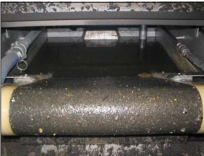
The screen is cleaned as it moves along the conveyor. The solids drop into a hopper. An optional hot water wash cleans grease and oil.
